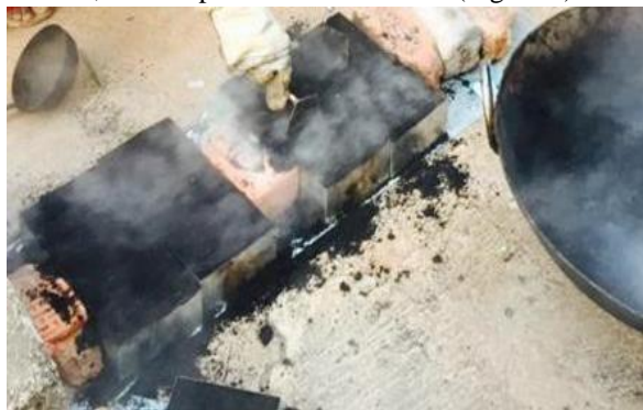
Fig.6: Releasing air bubbles from the mould by minor shaking and tamping
