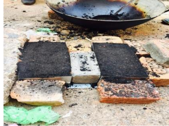
Fig.7: Set paver block just before demoulding
